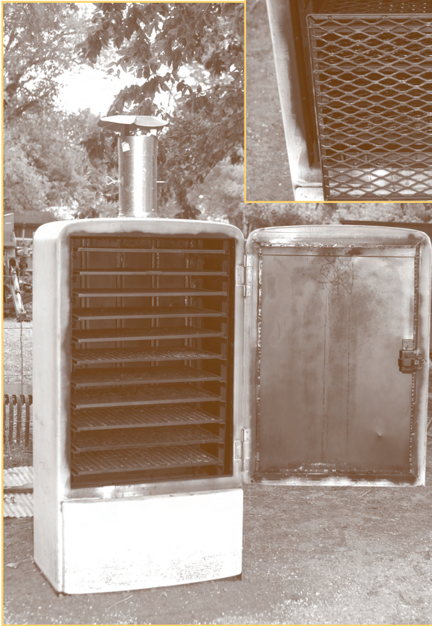
A shelving system was built and racks constructed of half-inch angle iron, and expanded metal provided enough area for up to 10 pounds of finished jerky.
